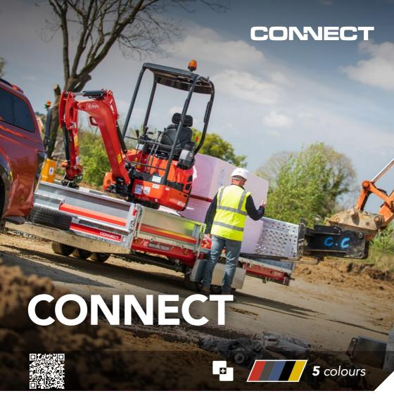
The Connect is a configurable utility trailer and is ideal for the transportation of construction materials and pallets as well as machinery and vehicles.
